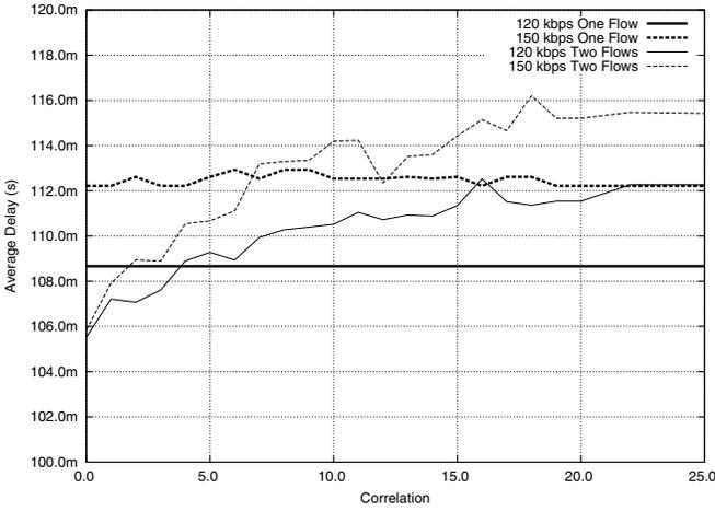
Fig. 10. Average end-to-end delay versus interference correlation. The delay increases with the correlation.
