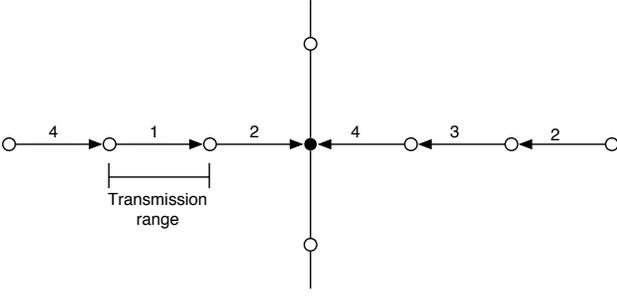
Fig. 3. Cross network topology. Data flows in to and out of the middle node. The edge labels show the optimal schedule for using two paths towards the middle node. The interference range is double the transmission range.
