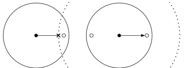
Fig. 1. Interfering transmissions in a chain of nodes. The transmission at the left hand side is unsuccessful due to the interference from the right hand transmission.
