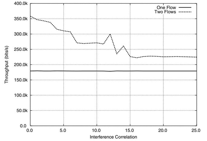
Fig. 11. Maximum aggregate throughput versus interference correlation. The throughput decreases with the correlation.
