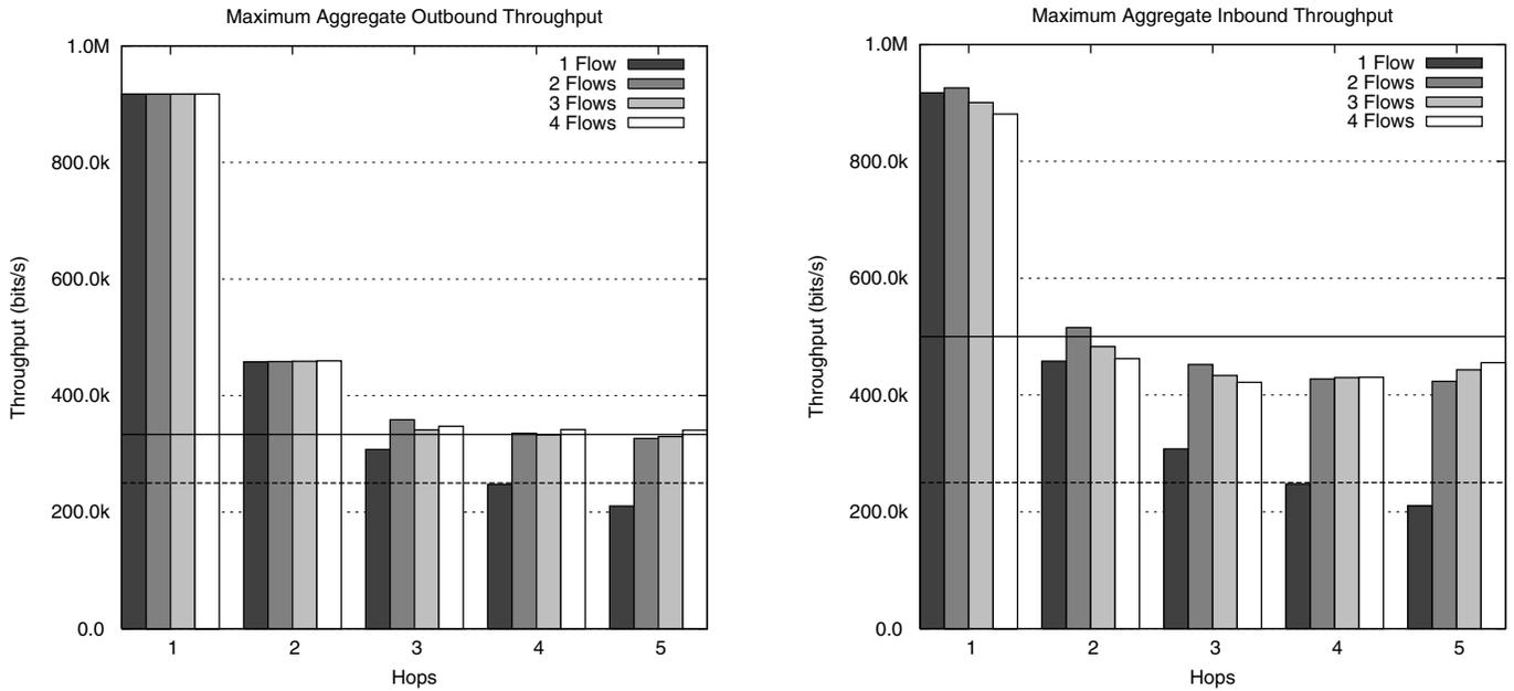
Fig. 8. Cross configuration maximum aggregate throughput. The solid lines mark the analytical multipath throughput for an infinite length chain with rate limiting, and the dashed lines indicate the analytical throughput for a single infinite length flow.
