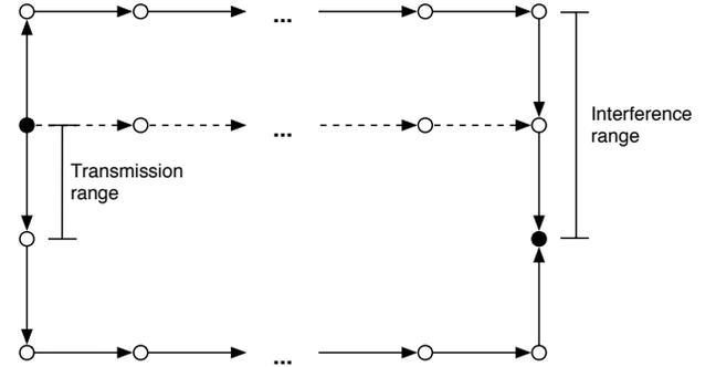
Fig. 5. Load balancing in a large grid network. The paths are forced away from the shortest path, shown with the dashed line, to ensure that the two paths are out of interference range of each other.
