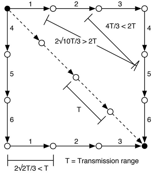
Fig. 4. The rate-limited transmission schedule for a simple  $4 \times 4$  grid topology.
