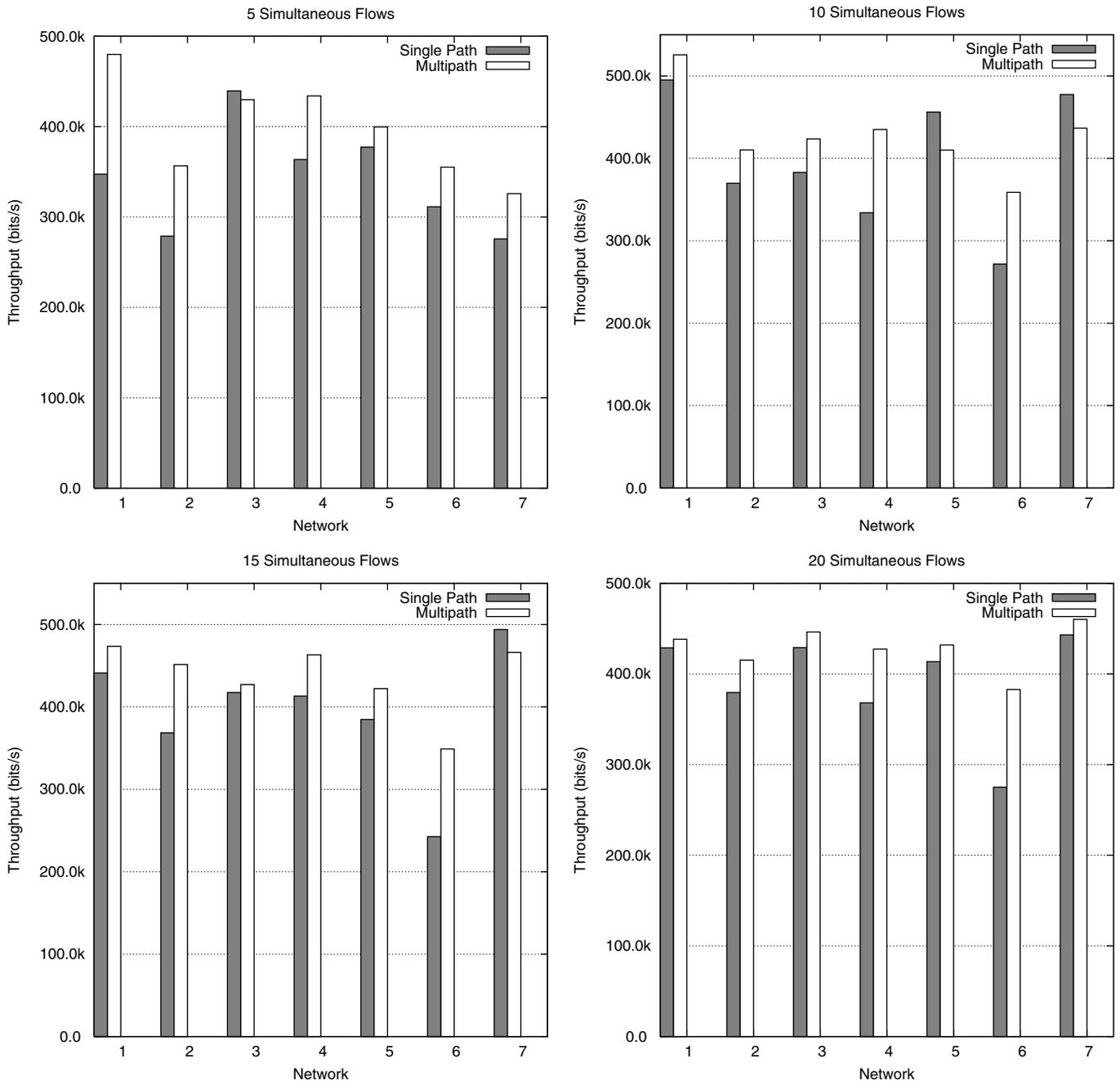
Fig. 13. Grid network aggregate throughput. This shows that using multipath routing can improve the aggregate throughput of grid networks in the majority of cases. It appears that multipath performance depends strongly on the traffic pattern, as all of these scenarios have the same topology, but use different paths.
