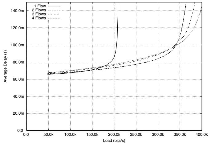
Fig. 9. Cross configuration five hop average end-to-end delay. When the throughput is low, more flows produces a larger delay due to the increase probability of collisions.
