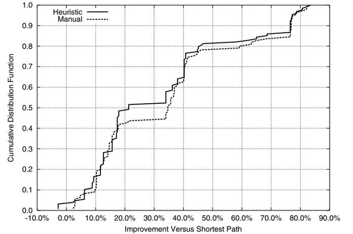
Fig. 12. Cumulative distribution function of the throughput improvement. The performance of the manual and the heuristic schemes is very similar.
