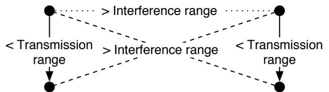
Fig. 2. Geometric requirements for simultaneous transmissions. If the inequalities are satisfied, both transmissions will succeed, according to the protocol model of interference. The dotted line represents an additional requirement for systems that use physical carrier sensing.
